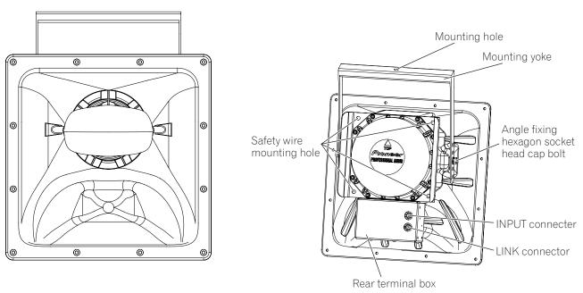
The XY-2 is a mid-high speaker taken from the mid-high range horn section of the XY-3B and can be used for various applications.
